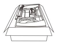
Step 3. Please insert the LSF ear and RSF ear to the back rest and make sure it is secured in position.
