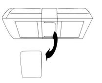
Step 3. Insert the LSF ear to the back rest and make sure it is secured in position.
