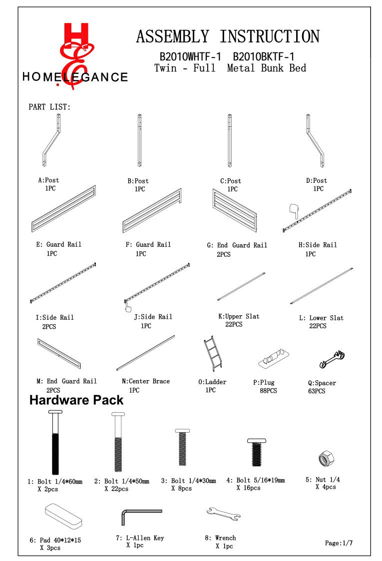
Note: Please do not tighten all bolts until the bed is assembled completely. STEP 1
