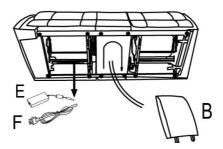
Step 2. Align the female brackets at the back onto the male brackets at the seat, insert and push to the end, make sure the brackets are secured in position.
