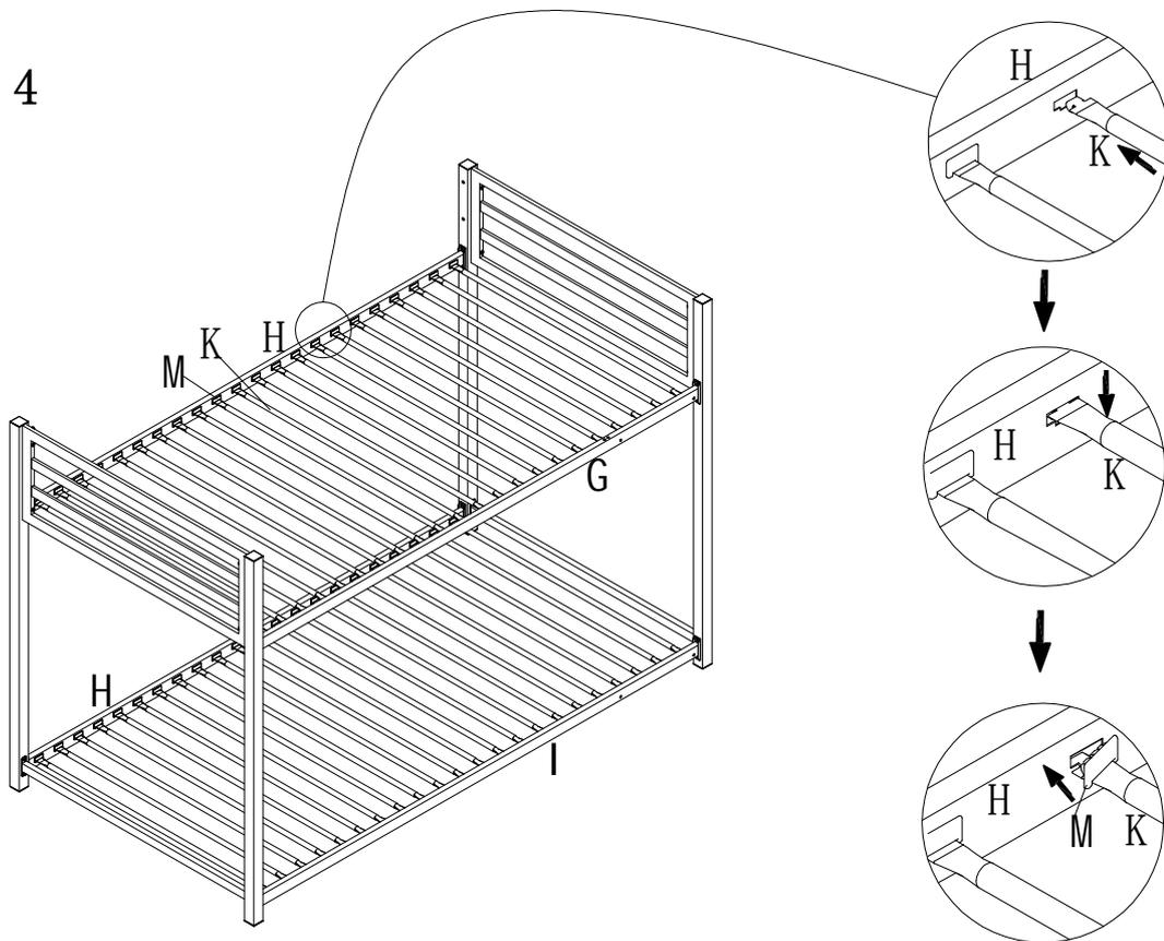
Note: Please do not tighten all bolts until the bed is assembled completely.
