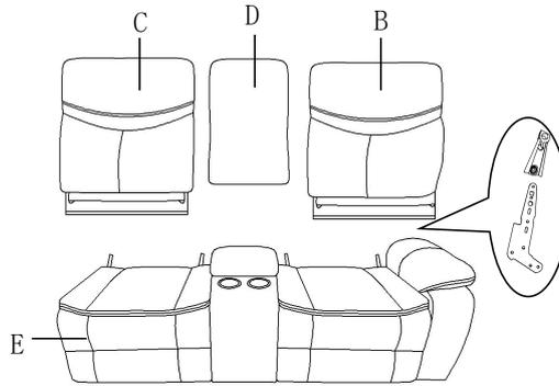
**Step 3. Insert the RSF ear to the back rest and make sure it is secured in position.**
