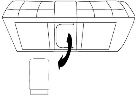
**Step 2. Align the female brackets at the back rest onto the male brackets at the seat, insert and push to the end, make sure the brackets are secured in position.**
