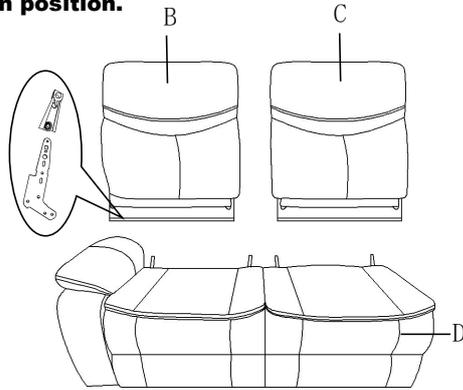
**Step 2. Insert the LSF ear to the back rest and make sure it is secured in position.**
