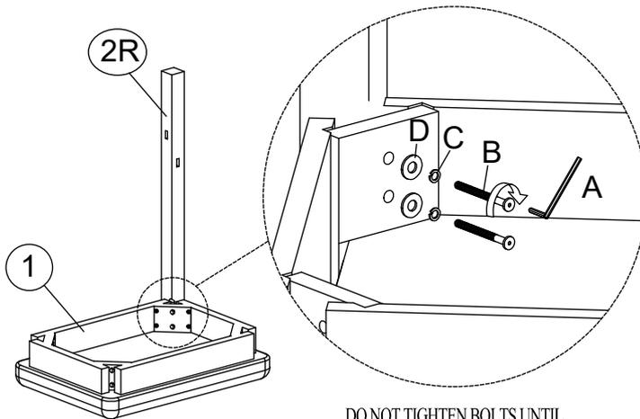
DO NOT TIGHTEN BOLTS UNTIL COMPLETELY ASSEMBLY /
