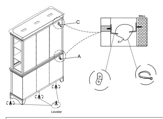
**NOTE:** Anti tipping hardware kit comes with this product. Please refer to the installation instruction ti the hardware pack. Anti-tipping hardware pack is located on the back panel
