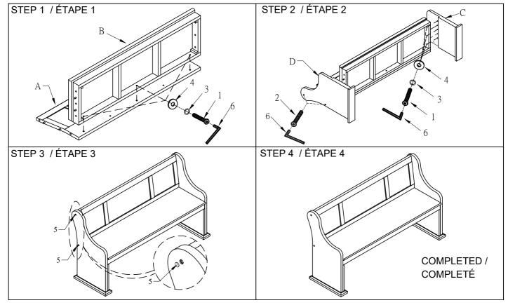
DO NOT TIGHTEN BOLTS UNTIL COMPLETELY ASSEMBLED.
