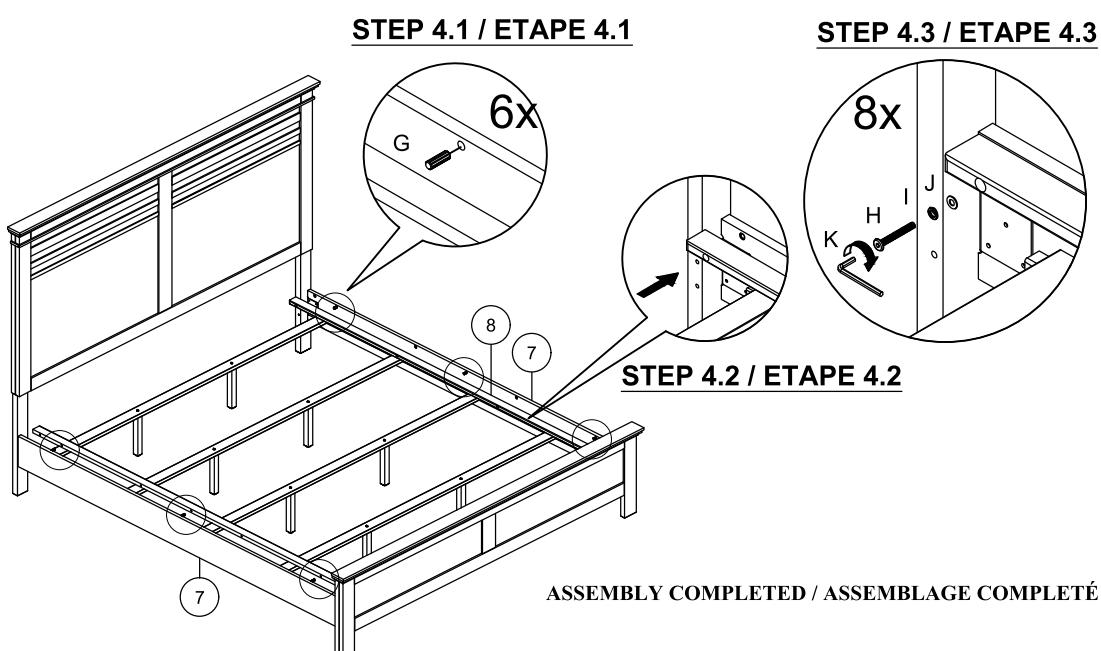
DO NOT TIGHTEN BOLTS UNTIL COMPLETELY ASSEMBLED.
