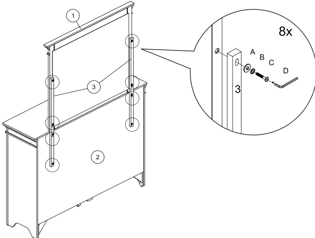
DO NOT TIGHTEN BOLTS UNTIL COMPLETELY ASSEMBLED.
