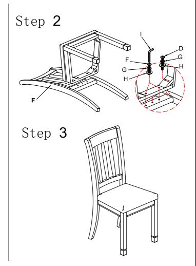
Do not tighten bolts until completely assembled.
