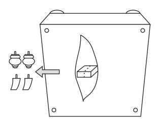
STEP #1: Align the legs to the bottom chair of the pre-drilled holes, rotate to tighten the legs.
