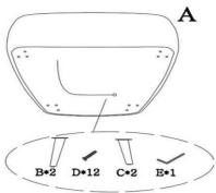
Step 2. Align the legs onto the pre-drilled holes at the bottom of unit, insert bolts then tighten with Allen key.
