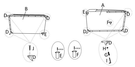
Step #3 Align and connect metal hooks to assemble the sectional.
