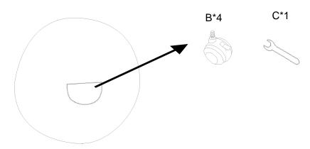
**Step 2.** Tighten the castors with Allen wrench by rotating the nuts **Step 3.Completed** at the end of the castors.
