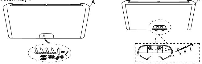
Step #3 Align the legs to the pre-drilled holes , insert the bolts then tighten with Allen key.
