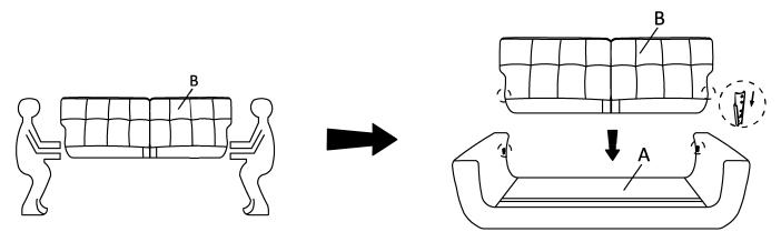
Step #2 Please lay down the back rest and take out legs and hardware for assembly. Align and insert the bolts go through the seat, tighten with Allen key .
