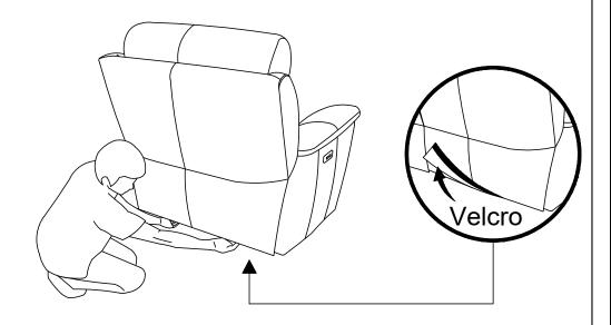
Step 2 To unlock the back of the recliner from its base, push up on the small metal hook built into the side of the recliner
