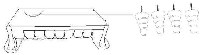
**Step#2** Align the legs to the pre-drilled holes as shown in drawing, rotate the legs in order to tighten it in secure and proper position.
