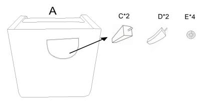
**Step 2.** Insert the washer onto the top of legs,rotate the legs to tighten it. Rear leg curves must face outward
