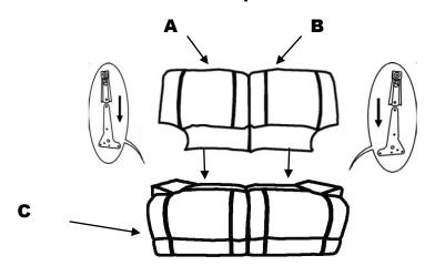
Step 2. Attach the arms to the both upper side of the seat, insert the arms and push to the end, make sure the brackets are secured in position.
