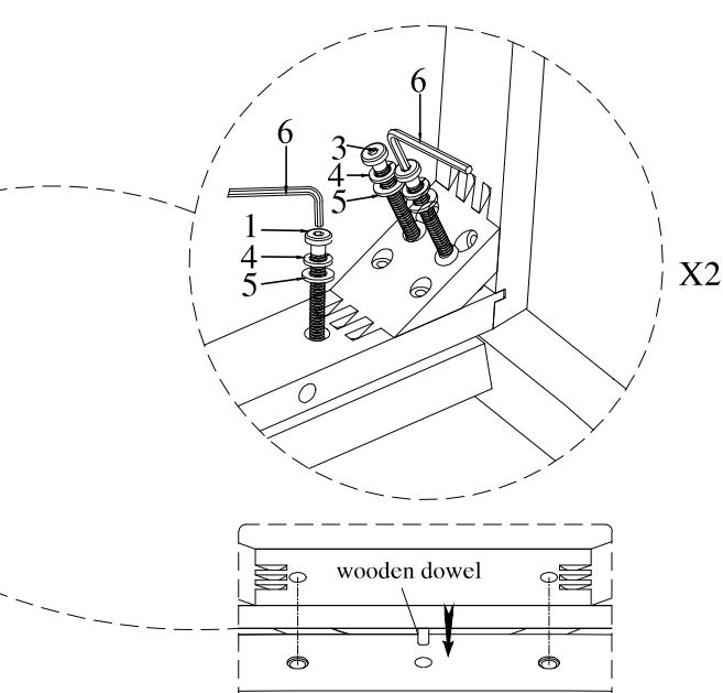
DO NOT TIGHTEN BOLTS UNTIL COMPLETELY ASSEMBLED.
