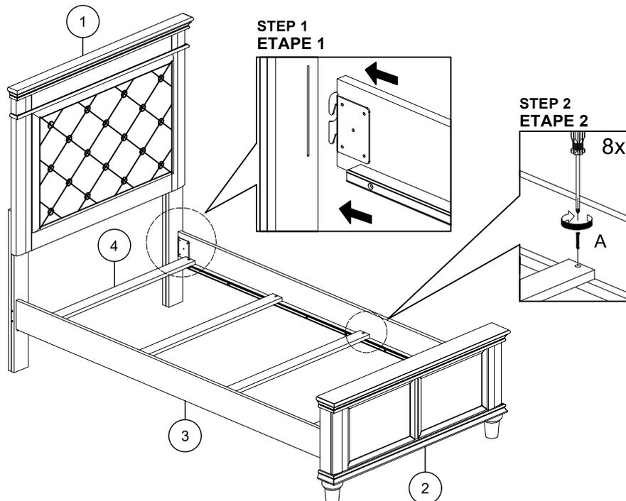
DO NOT TIGHTEN BOLTS UNTIL COMPLETELY ASSEMBLED.
